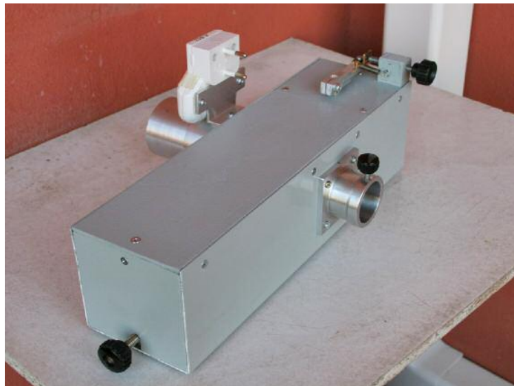
External view of the spectrograph built by Vittorio Lovato for the 500mm f/8 Ritchey-Chrétien telescope at the Libbiano Astronomy Centre.
